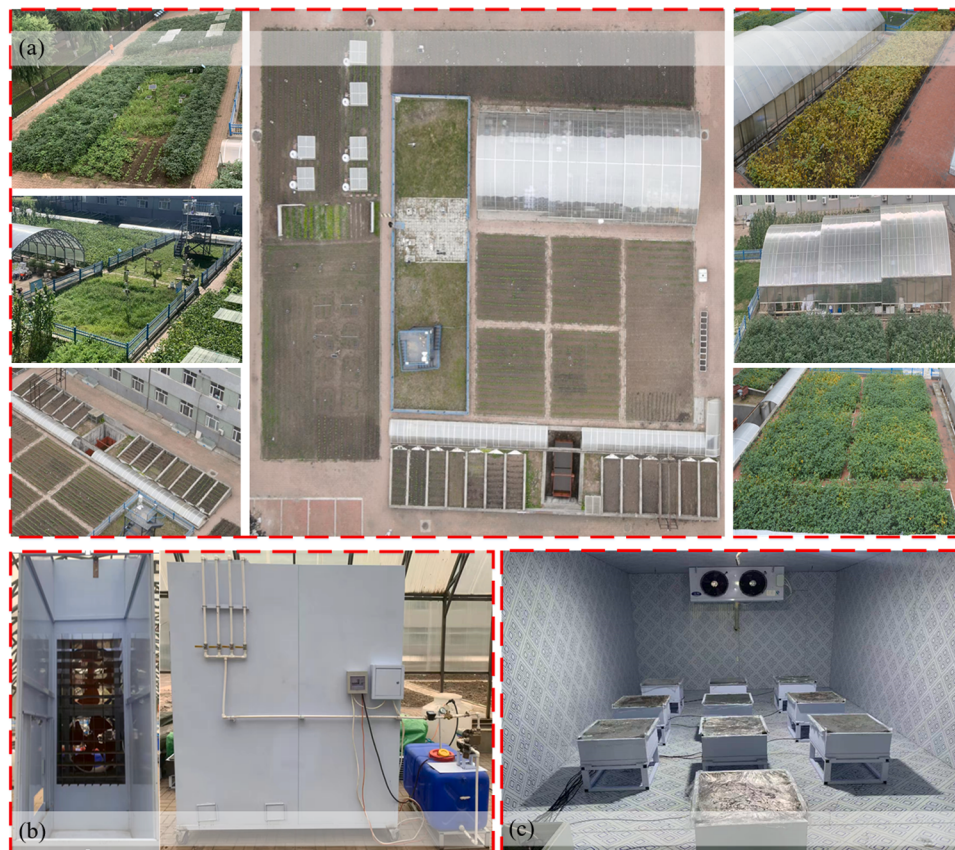
Fig. 1. Experimental site and installations diagram. (a) represents the experimental site, (b) denotes the wind tunnel-rainfall simulator, and (c) indicates the soil flume and artificial climate chamber.
