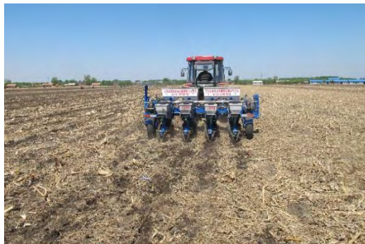
(c) 均匀垄免耕深松耕作技术模式 (c) Uniform ridge no-till deep tillage technology model
