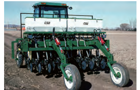
Figure 9. No-till grain drill developed at the Western Colorado Research Center at Fruita. Photo by Calvin Pearson
