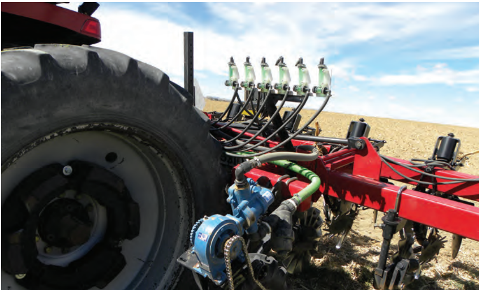
Figure 6. Strip till unit set up for deep placement of liquid fertilizer. Photo by Erik Wardle
