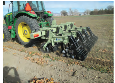
Figure 8. Four-row strip tiller used at WCRC-Fruita. Photo by Calvin Pearson
