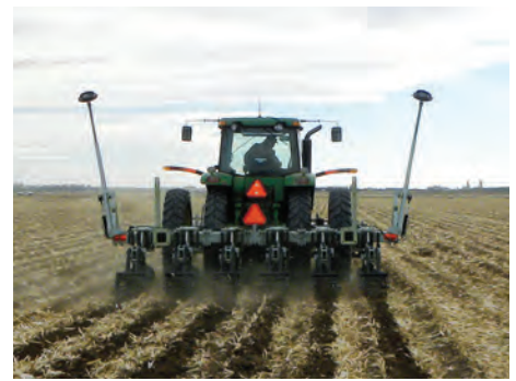
Figure 5. Strip till operation - proper adjustments to the implement are critical; keep in mind this is seed bed preparation, not rough tillage operation. Photo by Erik Wardle
